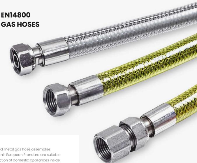
The corrugated metal gas hose assemblies according to this European Standard are suitable for the connection of domestic appliances inside or outside a dwelling using gas at a pressure lower than 0,5 bar. Gas hoses are suitable for 1st, 2nd and 3rd family gases. These gases are commonly refered to as manufactured gases, natural gases and liquid petrolium gases (LPG).
