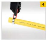
**D4.** Cut inner cover at **6th** Corrugation for **DN 15, DN20, DN25** and **DN32, 5th** Corrugation for **DN40** and **DN50** from the tubing end with a utility knife or with a hose peeler. Please pay attention to the number of corrugation.
