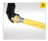
**D5.** Insert the tube into the fittings fimly until not seeing metal part of the tube.
