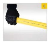
**D3.** Remove the cutter part outer sleeve by twisting and pulling it off the pipe from the cut end while firmly holding the other end with your other hand.
