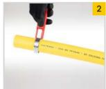
**D2.** Position the hose peeler onto the tube, making sure it's around 80 mm away from the cut end. Rotate it at least three times to slice through the outer layer while leaving the inner covering unharmed.
