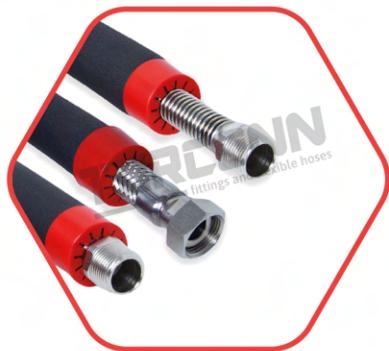
Fan coil hose assemblies provides reducing the transmission of noise and vibration that occur in fan coil systems. In addition, its flexibility allows for ease of installation and small movements caused by piping expansion. They are suitable for cold water and hot water systems.
